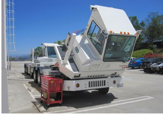
Rebuilt of a Kalmar Cargotec truck to electric truck
